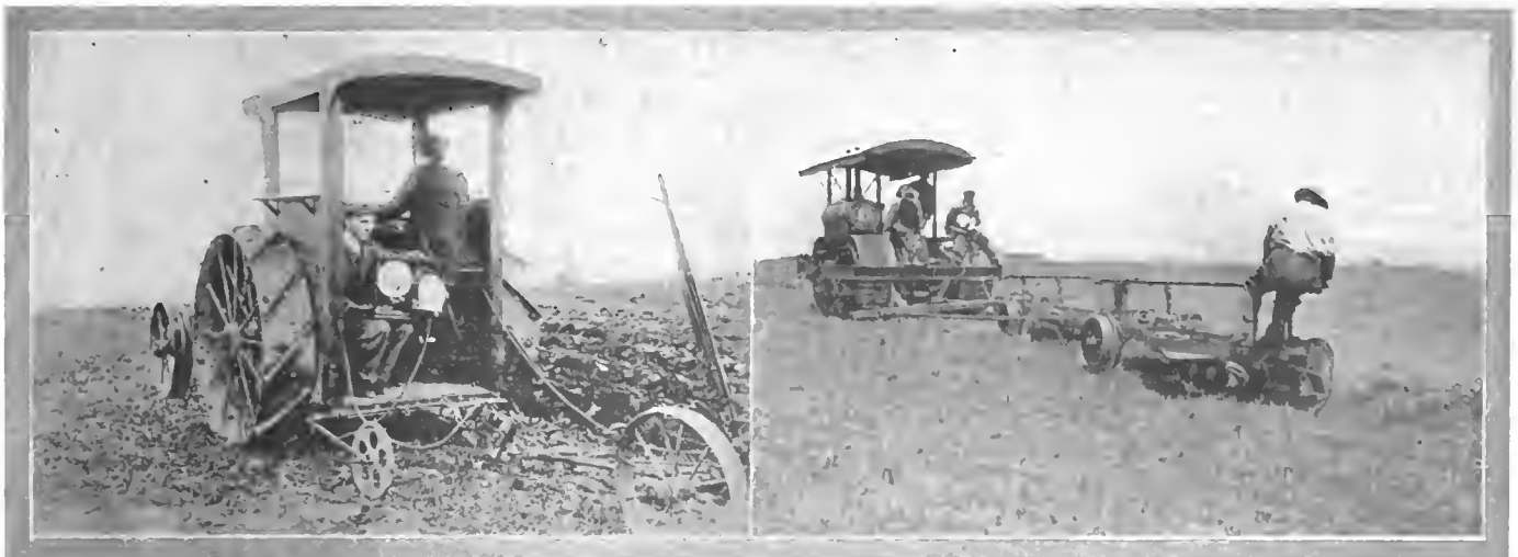
Hyatt hydrostatic instrument for measuring pull mounted on a tractor under actual service conditions
